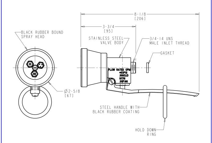
DIMENSIONS ARE IN INCHES AND [MILLIMETERS].
