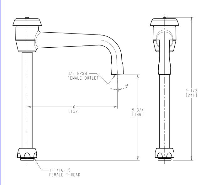
DIMENSIONS ARE IN INCHES AND [MILLIMETERS].
