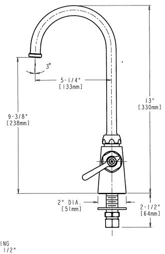
DECK MOUNTED SINGLE SINK FITTING GN2A RIGID/SWING GOOSENECK SPOUT
