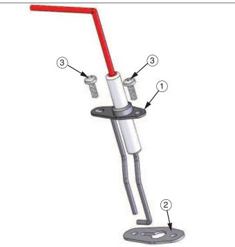
Fig. 1: Ignitor/Sensor Kit Components
