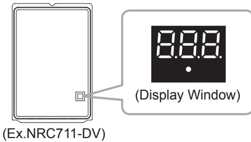
The display window allows you to view the status of unit or error codes.
