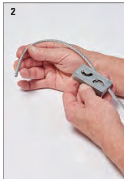
2 Loop wire rope through/around support
