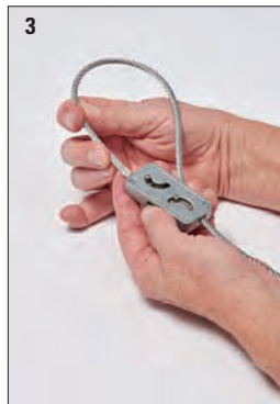
3 Pass wire rope back through KwikWire Clamp
