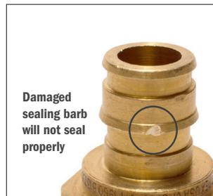
Damaged, cut or grooved barb on fitting.
