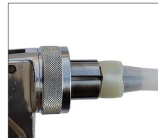
Failure to rotate tool inside tubing may cause unequal expansion. Remove any rings with unequal expansion.
