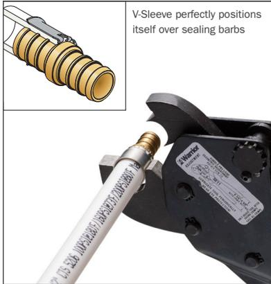
2. Compress tool perpendicular to tube - Compress only once. Remove any defective connections. Use a gauge to assure a proper joint. Test all completed joints.
