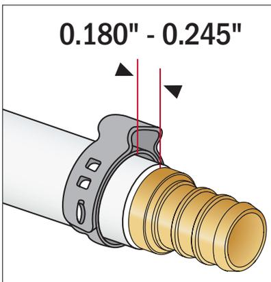
1. Cut tube at 90-degrees. Load clamp over tube end. Insert fitting fully into tubing. Position clamp between 0.180" and 0.245" from tube end.
