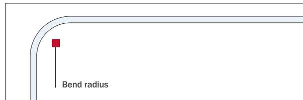
If coiled tubing is being used and the bend direction is against the coil direction, multiply noted bend radius by a factor of 3. Warmer tubing bends more easily. Generally a bend radius of 8x tube diameter should be sufficient. Using a manufactured PEX bend support will aid in assuring the proper bend radius.
