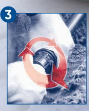
Position collet and nut, then turn to tighten. The fitting is fully installed when the nut can't be tightened further.
