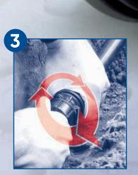
Tighten the nut with a turn of the hand and then firmly with a wrench.
