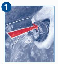
Assembly is so easy you can even do it under live conditions. Cut the pipe square and line up the pre-assembled fitting.
