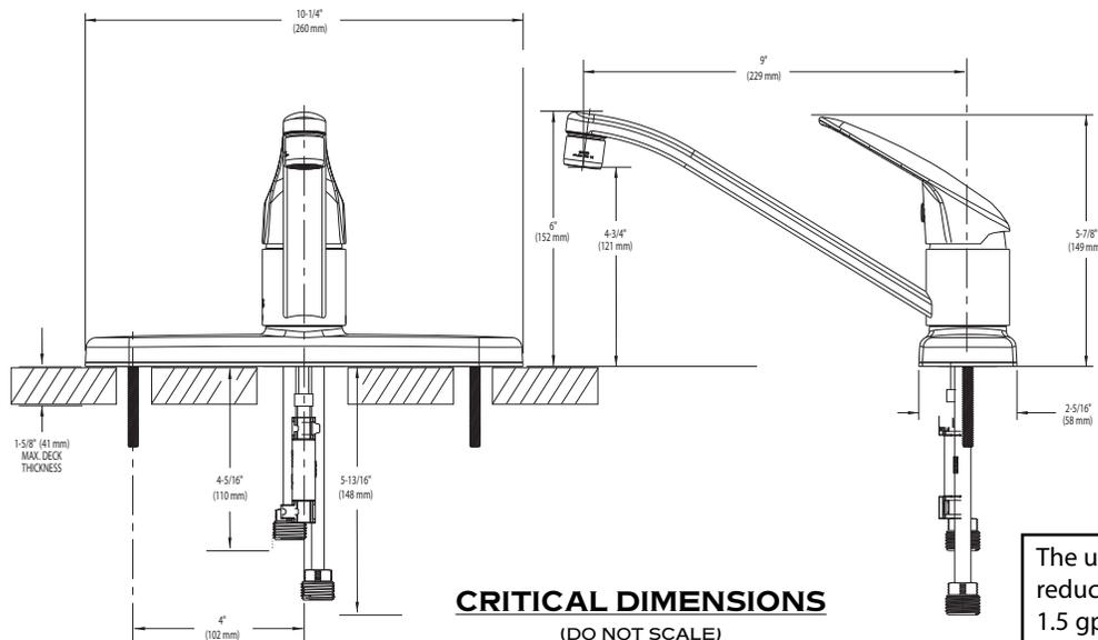
The use of aerator part 116711 reduces flow to a maximum of 1.5 gpm (5.7L/min.)
