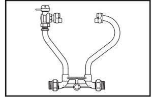
FULL PORT ANGLE BALL VALVE BY METER NUT (1" METER)
