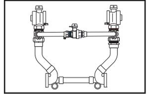
FLANGED ANGLE BALL VALVE BY FLANGED ANGLE BALL VALVE WITH HIGH BY-PASS (2" METER)
