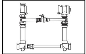
ANGLE KEY VALVE BY ANGLE DUAL CHECK VALVE (2" METER) WITH HIGH BYPASS BALL VALVE
