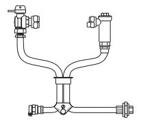
ANGLE BALL VALVE BY ANGLE DUAL CARTRIDGE CHECK VALVE (1" METER)
