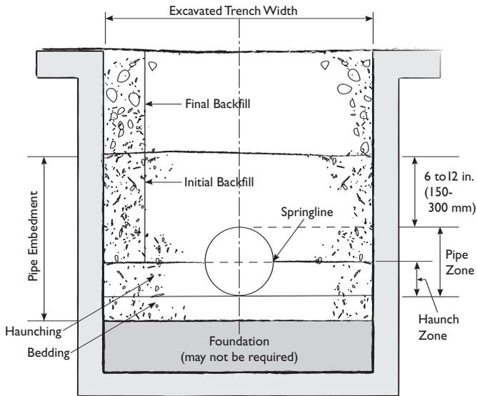
**Depth of Burial for GF Harvel PVC Pipe:** When installed underground an external load is placed on a PVC Pipe, its diameter will begin to deflect, meaning its sides will move outward and slightly downward. If GF Harvel PVC pipe is buried in supportive soil, the stiffness of the soil will help support the pipe. This action and reaction is the key to how a PVC pipe carries external loads while buried.
