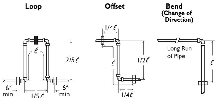
Hangers or guides should be free of rough or sharp edges and should only be placed in the loop, offset, or change of direction as indicated above. Piping supports should restrict lateral movement and should direct axial movement into the expansion loop. Do not restrain "change in direction" configurations by butting up against joists, studs, walls or other structures.
