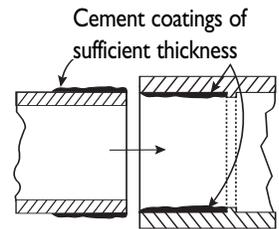
If the cement coatings on the pipe and fittings are wet and fluid when assembly takes place, they will tend to flow together and become one layer. Also, if the cement is wet, the surfaces beneath them will still be soft, and these softened surfaces in the tight part of the joint will tend to fuse together.
