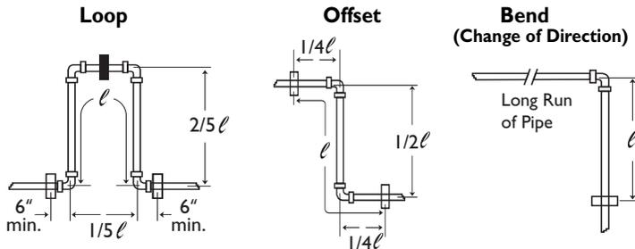
Hangers or guides should only be placed in the loop, offset, or change of direction as indicated above, and must not compress or restrict the pipe from axial movement. Piping supports should restrict lateral movement and should direct axial movement into the expansion loop configuration. Do not restrain "change in
