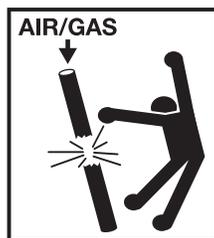
Use of compressed air or gas in PVC/CPVC pipe and fittings can result in explosive failures and cause severe injury or death.
