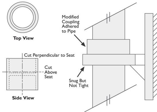
water lines, to minimize deflection caused by thermal expansion. The guidelines provided herein for vertical risers do not apply to horizontal runs. For horizontal runs, the use of expansion loops, offsets, bends, and other means are recommended to compensate for movement due to changes in temperature. Refer to Thermal Expansion and Contraction section for additional information. Contact GF Harvel Technical Services for additional information if necessary.
