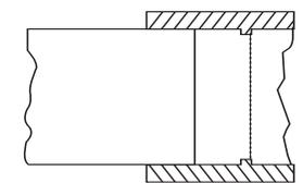
As the solvent dissipates, the cement layer and the softened surfaces will harden with a corresponding increase in joint strength. A good joint will take the required working pressure long before the joint is fully dry and final strength is obtained. In the tight (fused) part of the joint, strength will develop more quickly than in the looser (bonded) part of the joint. Information about the development of bond strength of solvent cemented joints is available.
