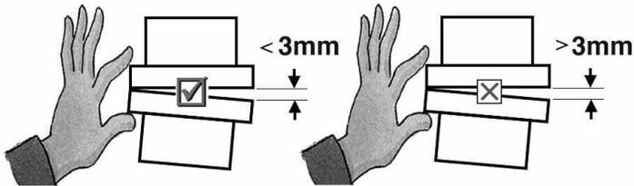
If the gap between the components cannot be closed by pinching them with one hand, or if the angle between them is too large, refit the system with proper alignment before bolting.
