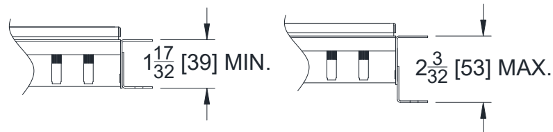
ANCHORING SUPPORT LEG ADJUSTMENT RANGE
