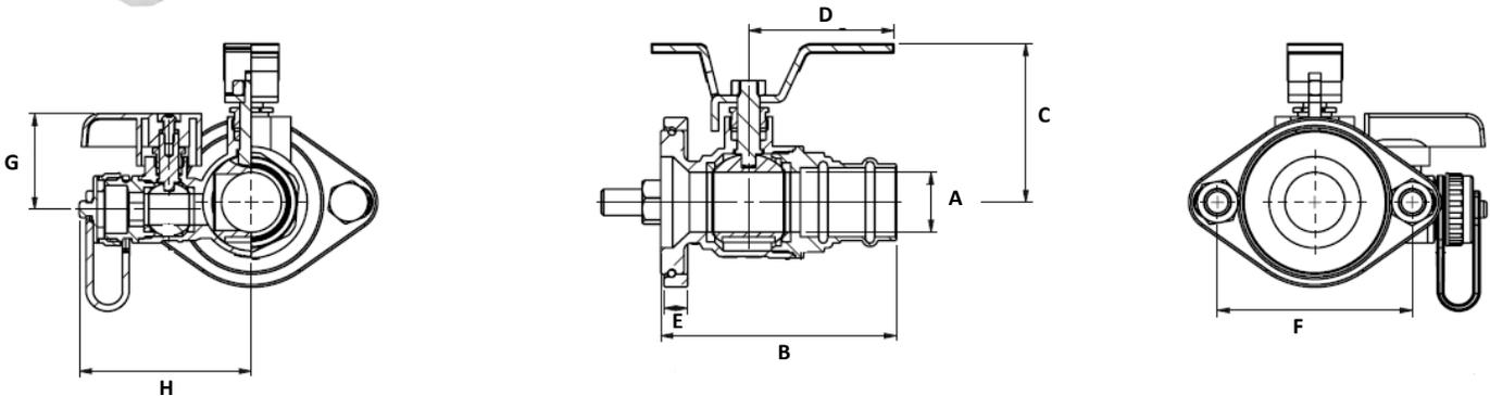
**Specifications:** Designed for residential, commercial or industrial use with water only. This approved Webstone valve is actuated by a blowout proof stem and features an adjustable packing gland. HV models fit both standard and high velocity pumps.
