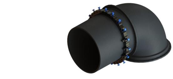
4. Push the One-Lok gland toward the fitting and center it around the pipe with the lip evenly against the gasket.
