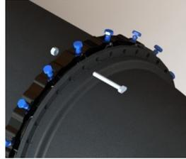
6. Tighten the nuts in an alternate method (STAR PATTERN) to the recommended torque of 45-60 ft-lbs for 3", 75-90 ft-lbs for 4" – 24", 100-120 ft-lbs for 30", 36", 120 – 150 ft-lbs for 42", 48", 54", 60" & 64" sizes, use of a torque indicating wrench is recommended to confirm the applied torque.
