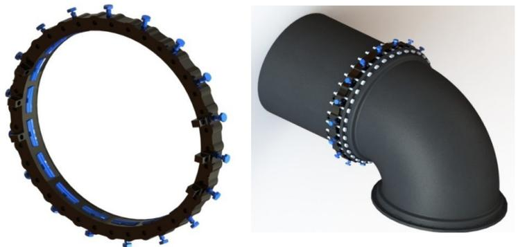
1. Clean the fitting socket & pipe end. Lubricate mechanical joint gasket & pipe end with soapy water or approved lubricant meeting AWWA C111/A21.11. (A transition gasket is required if using on steel OD pipe)
