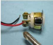
Drill a 5/8" hole in the face of the cabinet where the D'MAND KONTROLS® pump is installed. Next, feed the two wire cable through the 5/8" hole; connect the hard-wired button to the two lead cables. (Red and Black) The hard-wired button has two (2) terminals to affix a wire on each side.
