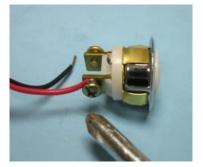
Drill a 5/8" hole in the face of the cabinet where the D'MAND KONTROLS® pump is installed. Next, feed the two wire cable through the 5/8" hole; connect the hard-wired button to the two lead cables. (Red and Black) The hard-wired button has two (2) terminals to affix a wire on each side.
