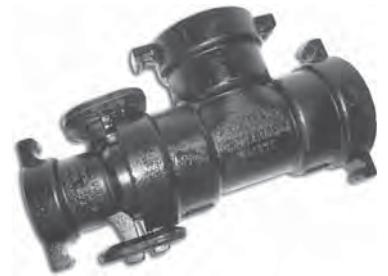
Shown is an assembled 3 x 2 x 3 tee. The 3 x 2 reducer is installed and restraint rings have been latched over the lugs to create an assembled fitting.
