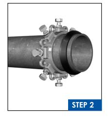
Brush both the gasket and the plain end of pipe with soapy water or approved pipe lubricant, which meets ANSI/AWWA C111/ A21.11. Slide the MJ gasket over the pipe with beveled edge towards the pipe end.
