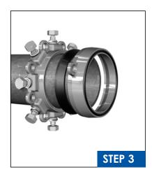
Insert 7200 ring onto the pipe with O-Ring facing the flange component. O-Ring has been glued in place at the factory.
