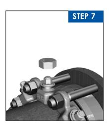
Continue tightening the bolts in an alternate manner until torque off bolt heads twist off. If removal is necessary, use 5/8 inch hex head provided. If reassembly is required, assemble the joint in the same manner following steps 1 to 6 and tighten wedge bolts to 90 ft-lbs.
