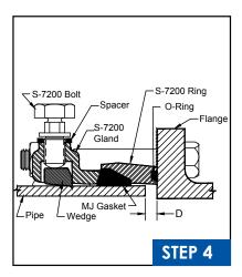
Move the pipe towards the flange face bringing it within max. allowable distance "D" from flange face. Refer to Table A for max. allowable distance "D" and Max. allowable deflection of pipe.
