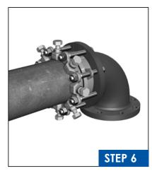
Tighten torque off bolts in an alternate manner such that all wedges touch the pipe. Never turn a single bolt over 180 degrees without alternating to another bolt.
