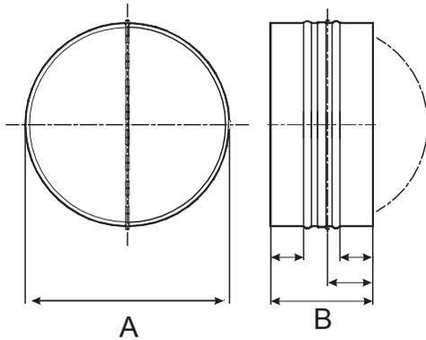
Backdraft dampers are designed with galvanized steel collars and have lightweight aluminum damper blades. They are spring loaded for positive closure.
