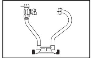
FULL PORT ANGLE BALL VALVE BY METER NUT (5/8" X 3/4" METER)
