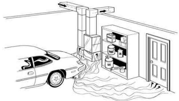
FIGURE 2 MIGRATION OF DANGEROUS SUBSTANCES, FUMES, AND ODORS INTO LIVING SPACES
