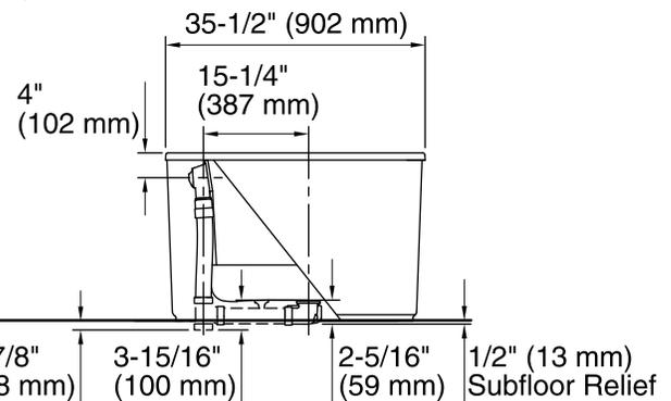
\* Allow for appropriate relief in subfloor for drain clearance.
