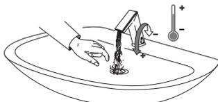
Optional — To fix temperature, set lever to the desired position, then remove lever and plug hole with Cap.
