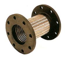
Style SECF Stainless Steel Braided Pump Connectors are manufactured using 300 alloy stainless hose and braid and a steel plate with 150# drilling as the flange. Other end fittings, including 300# flanges and grooved nipple ends, are available. Working pressures up to 315 psi at 250°F. Standard and special lengths are available. Standard sizes range from 2" through 16" I.D.
