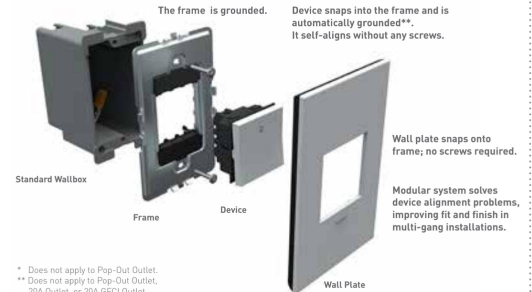
Devices simply snap into the frame from the front. During installation, screw the frame to the box, then pull the wires through the frame and wire the device. Then, simply snap the device into the frame.
