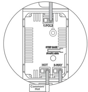
**NOTE** - In a 3-Way installation, use one dimmer and one switch. Do NOT use two dimmers.
