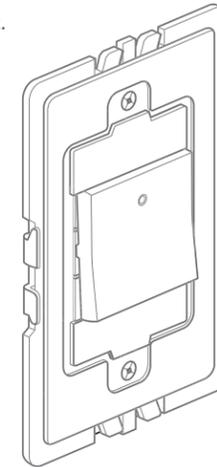
NOTE - If you need to remove switch after snapping into frame, first remove frame from wall box to access the three locking tabs on the back of the switch. Insert a flat screwdriver to depress tabs as you apply pressure to push switch out.
