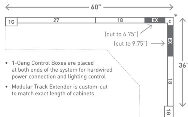
**Sample Installation:** Direct wire with system controls in a remote location
