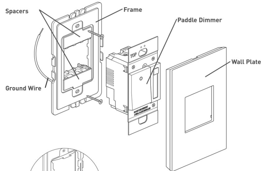
**Remove spacers from the frame.** Since this dimmer fills the frame completely, you will not need the spacers. From the back of the frame, pinch the tabs on the spacer to release.
