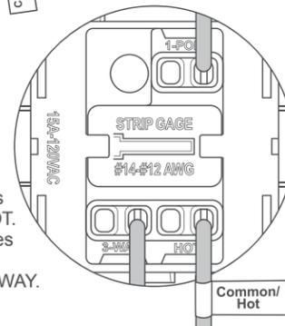
**5** Carefully fold wires into box. Snap switch into frame.
