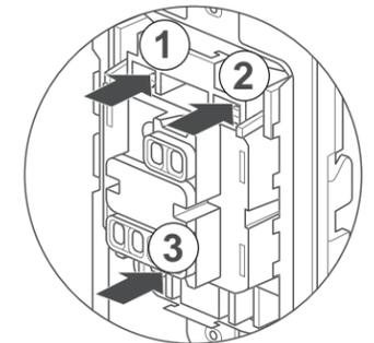
**6** Snap wall plate to frame. There are three click-stops to adjust the fit of the wall plate to the switch and the wall.
