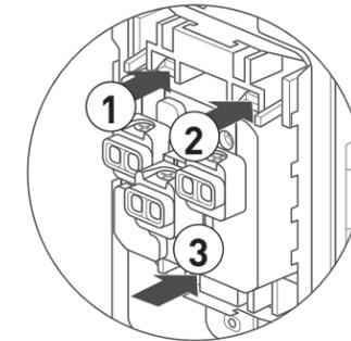
**6** Snap wall plate to frame. There are three click-stops to adjust the fit of the wall plate to the outlet and the wall.
