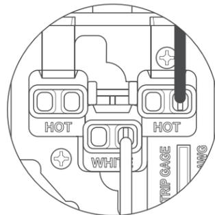
**⚠ WARNING:** Do not pair different size wires in the same terminal. If you have different size wires, use a wire nut to add a 6 inch pigtail of the same gauge wire to the smaller gauge wire.
