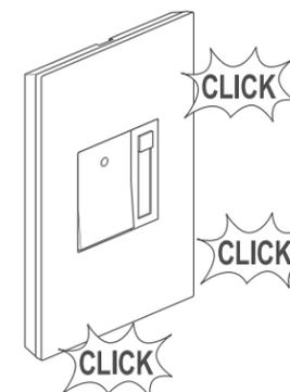
**NOTE** - To remove wall plate, insert a small, flat screwdriver in notches on wall plate and twist gently to pry from frame.
