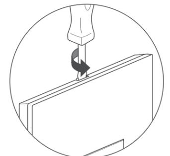
NOTE - To remove wall plate, insert a small, flat screwdriver in notches on wall plate and twist gently to pry from frame.
