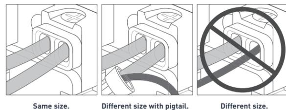
**5** Carefully fold wires into box. Snap outlet into frame.
