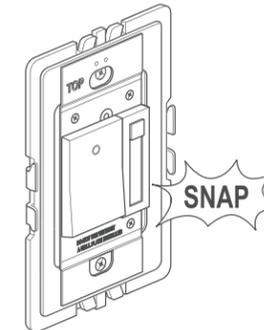
**NOTE** - If you need to remove dimmer after snapping into frame, first remove frame from wall box to access the four locking tabs on the back of the dimmer. Insert a flat screwdriver to depress tabs as you apply pressure to push dimmer out.
