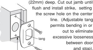
the screw hole on the center line. (Adjustable tang permits bending in or out to eliminate excessive looseness between door and stop).
