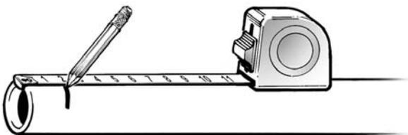
**STEP 4** Insert pipe all the way to mark. Pipe should bottom out at the pipe stop.
