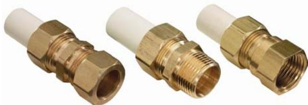
Standard compression fittings with brass or plastic ferrules can be used. However, PTFE tape should be applied over the brass ferrule to compensate for the dissimilar thermal expansion rates between the brass and CPVC.
