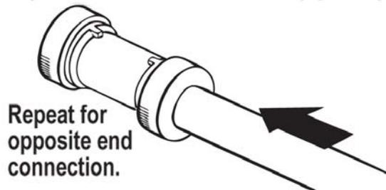
**WARNING: DO NOT INSERT FINGERS. ENSURE THAT PIPE AND FITTINGS ARE FREE OF DIRT AND DEBRIS PRIOR TO INSTALLATION.**
