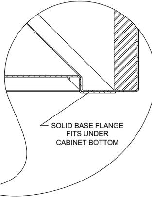
1. REMOVE 2 SCREWS, LIFT BASE UP, SLIDE FORWARD TO REMOVE.
