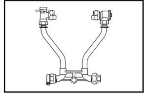
ANGLE KEY VALVE BY ANGLE CHECK VALVE (1" METER)
