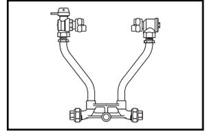
ANGLE BALL VALVE BY ANGLE CHECK VALVE (5/8" METER)
