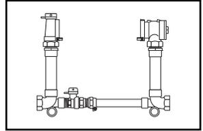
ANGLE KEY VALVE BY ANGLE DUAL CHECK VALVE (1-1/2" METER) WITH BYPASS BALL VALVE
