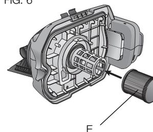
3. Clean the filter by shaking off excess dust, tapping into a waste receptacle, then rinsing under running water. Depending on the condition of the filter, a water wash is not always required. Do not use a brush to clean filter.
