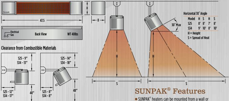
SUNPAK<sup>®</sup> Heaters are available with single or dual stage control systems, and casings are available in black or stainless steel finishes. The decorative face trim is available in black, bronze or stainless steel and will fit on all SUNPAK<sup>®</sup> models. SUNPAK<sup>®</sup> heaters are available in S25 – 25,000 Btu/Hr and S34 – 34,000 Btu/Hr.
