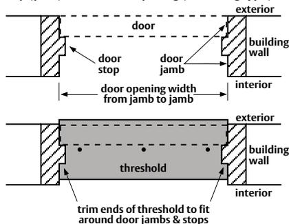
1. Measure width of door opening from jamb to jamb and stop to stop and mark ends of threshold for trimming.
