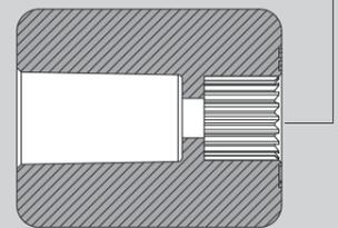
**3** Confirm that Valve is in the "Off" position. Place appropriate Connector on to the Spindle of the Valve, making sure to orient the Connector so that one set of Splines are in a perfectly vertical position.
