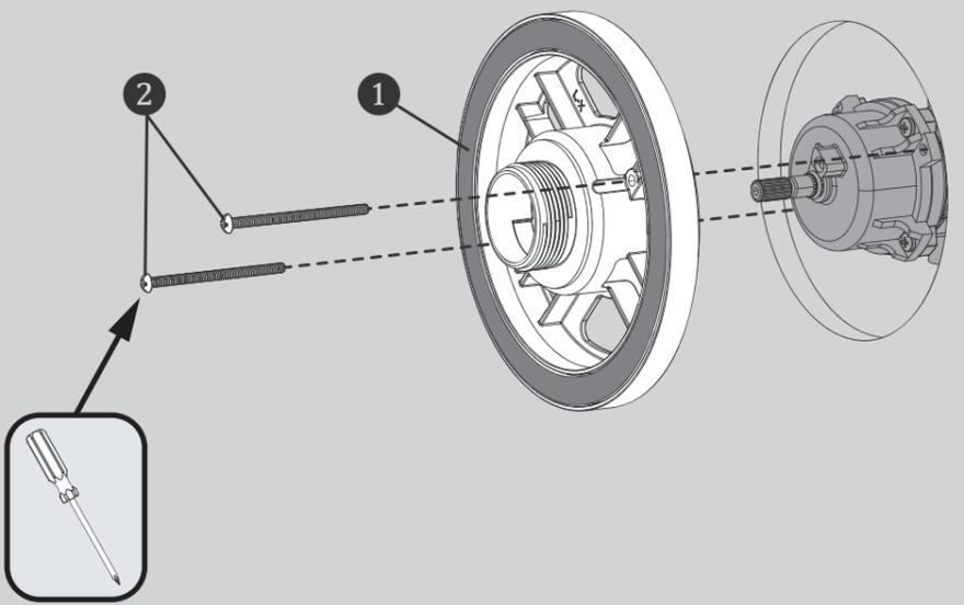
**2** There are two connectors included to allow for both Shallow Mount (Valve Centerline is 2.5"-3.0" from finished wall surface) and Deep Mount (Valve Centerline is 3.0"-3.5" from finished wall surface) applications. Please select Connector appropriate for your installation.
