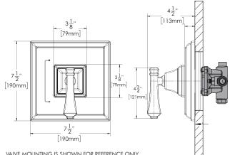
VALVE MOUNTING IS SHOWN FOR REFERENCE ONLY. VALVE IS NOT INCLUDED WITH CPT-8001-P
