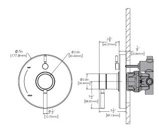
VALVE MOUNTING IS SHOWN FOR REFERENCE ONLY. VALVE IS NOT INCLUDED WITH CPT-1400-P / CPT-1400-KN
