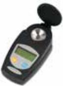
The **Palm Abbe** refractometer is fast, convenient, and easy to use. Simply place a drop or two of fluid in the titanium well and press a button. The custom-designed microprocessor is temperature compensating and delivers readings for glycerine and propylene glycol for both percentage by volume and freeze point. Accuracy of +/- .10 % .
