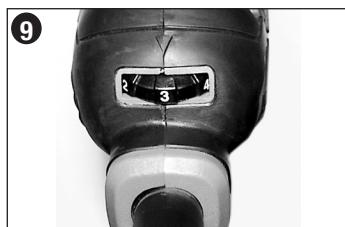
The numbered positions, 1 through 6 inscribed on the variable speed dial, do not indicate any precise speed but are good reference points. The higher the number, the higher the tool speed.
