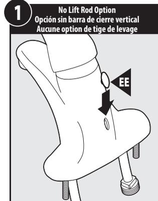
For Faucet installed without Lift Rod (D or Q): Insert Plug Button (EE) into slot in Faucet Body.
