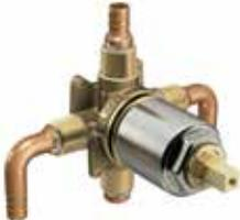
Shower valve – <b>Pressure-balancing</b> in-wall valve without shut-off stop <ul style="list-style-type: none"> <li>• <b>This item must be purchased in case quantity of 12</b></li> <li>• Inlets – 1/2" PEX adapters, 90° elbow, pointing down</li> <li>• Shower outlet – 1/2" PEX adapter, straight</li> <li>• Tub outlet – brass plug</li> <li>• Ceramic disc cartridge</li> <li>• Temperature control with flow control</li> </ul>       | 12        | 2.79         |
