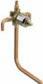
Tub/Shower valve – <b>Pressure-balancing</b> in-wall valve without shut-off stop <ul style="list-style-type: none"> <li>• <b>This item must be purchased in case quantity</b></li> <li>• Inlets – 1/2" PEX adapters, 90° elbow, pointing down</li> <li>• Shower outlet – 1/2" PEX adapter, straight</li> <li>• Tub outlet – 8" x 7" copper tube</li> <li>• Ceramic disc cartridge</li> <li>• Temperature control with flow control</li> </ul> | 12        | 3.24         |
