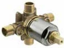
Tub/Shower valve – <b>Pressure-balancing</b> in-wall valve with temperature limit stop <ul style="list-style-type: none"> <li>• Combination 1/2" male IPS/CC connections</li> <li>• Ceramic disc cartridge</li> <li>• With shut-off stops and check valves</li> <li>• Temperature control with flow control</li> </ul>                                                                                                                        | 12        | 2.78         |
