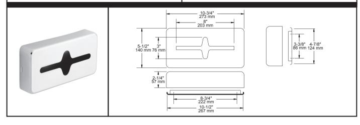
MATERIALS: Base Wall Panel - 20 Gauge, Galvanized Steel
