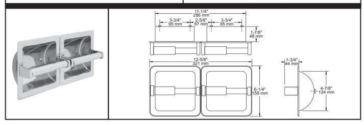
MATERIALS: Stainless steel recessed shells are stamped from 22 gauge corrosion resistant type 304 stainless steel and are polished or satin.
