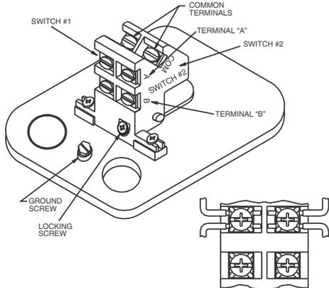
BREAK WIRE AS SHOWN FOR SUPERVISION OF CONNECTION. DO NOT ALLOW STRIPPED WIRE LEADS TO EXTEND BEYOND SWITCH HOUSING. DO NOT LOOP WIRES.
