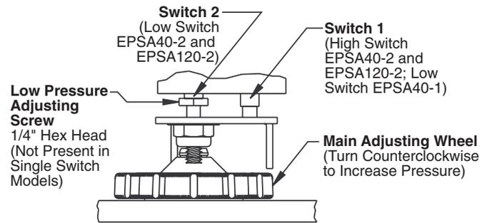
**NOTE:** Each 1/2 turn of Low Pressure adjusting screw adjusts pressure approximately 5 psi. Turn counter clockwise to increase pressure. Turn clockwise to decrease pressure. Each 1/2 turn of High Pressure adjusting wheel adjusts pressure 11 psi on the EPS40-2 and 40 psi on the EPS120-2.
