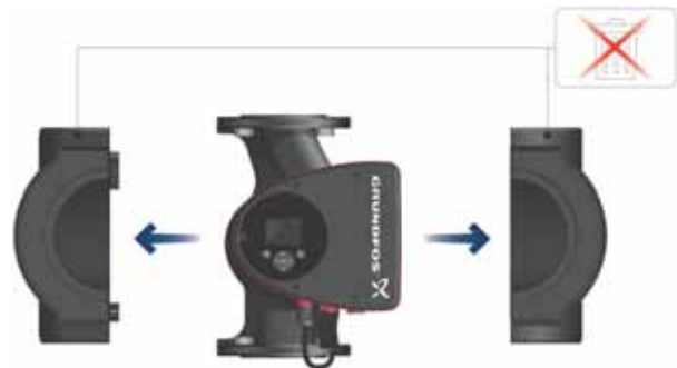
Fig. 3 Fitting insulating shells to the pump
