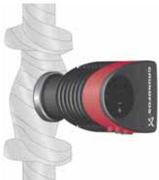
Fig. 13 Insulation of pump housing and pipework
