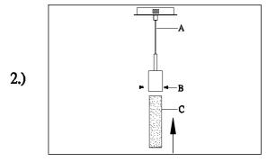
Step.2: Install glass into holder using 2 screws supplied
