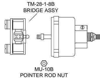
6. To disassemble bridge assembly, see drawing next page (remove TM25-3A holder nuts with screwdriver in slots provided).
