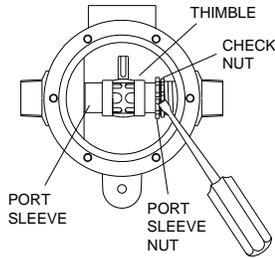
6. To clean thermostat group, remove coil sleeve stud and take off thermostat group.
